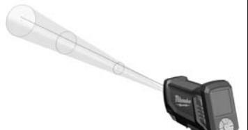
a - Distance laser point to center of spot temperature area (18 mm)
