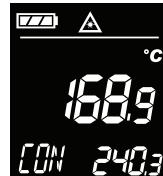
2. The display will continue to update the contact temperature (CON) while the temperature probe reaches thermal equilibrium with the object being measured. The display will shut off after about 20 min.
