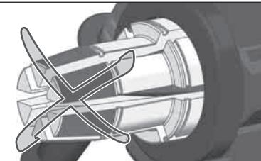
Clean the expander cone with a clean, lint-free cloth and then apply a thin coat of lubricant to the expander cone.
