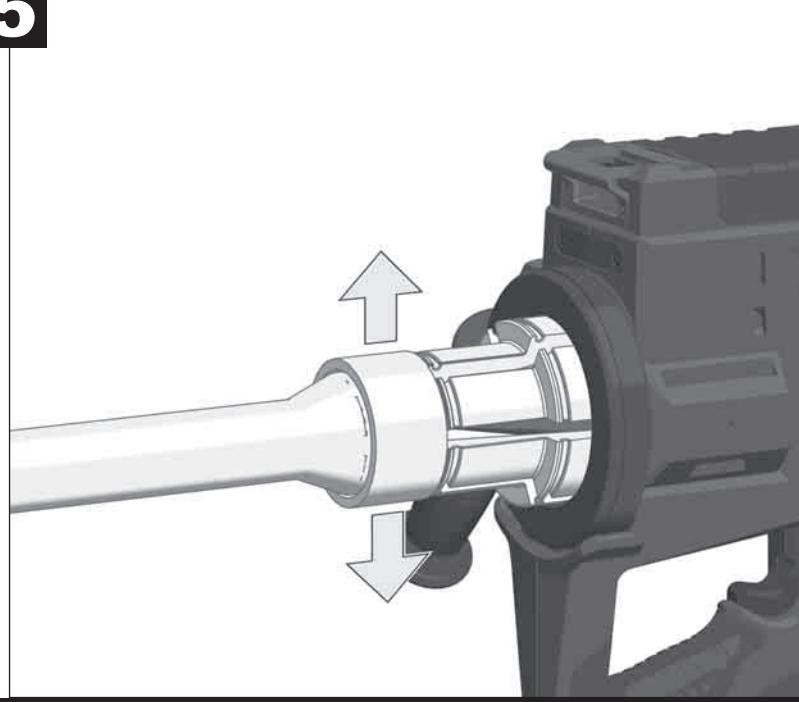
The tube will expand automatically. To cancel quickly, pull and release trigger.
