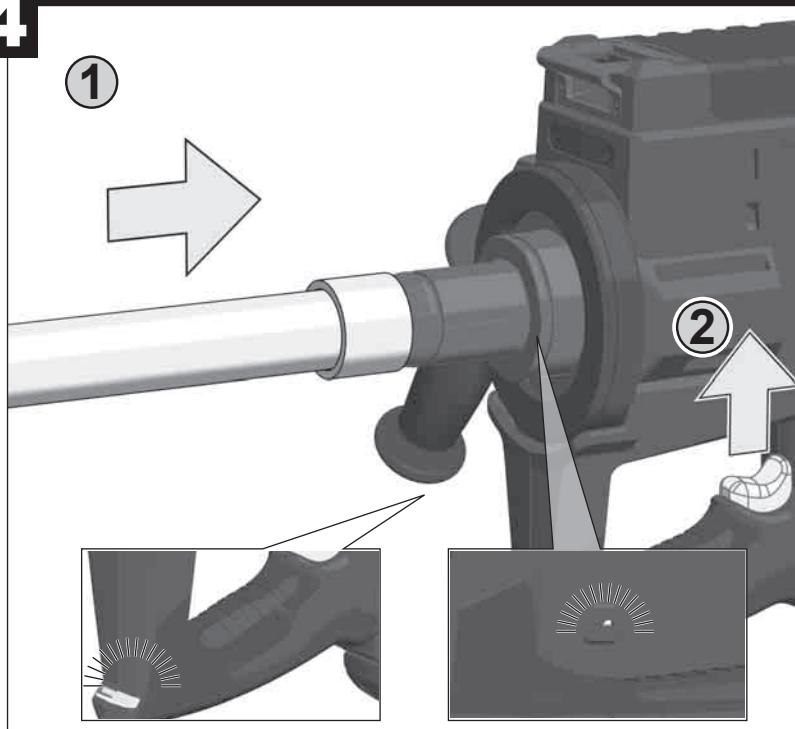
Pull and hold the trigger to initiate the rotation of the expander head. Do not insert into the tubing!
