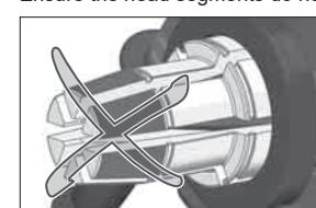
Rotate the six expander segments in the clockwise direction. The head will rotate freely. The head should not rotate counterclockwise.
