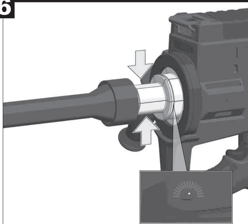
When the expander reaches maximum diameter it will automatically retract and the green LED blinks 3 times.
