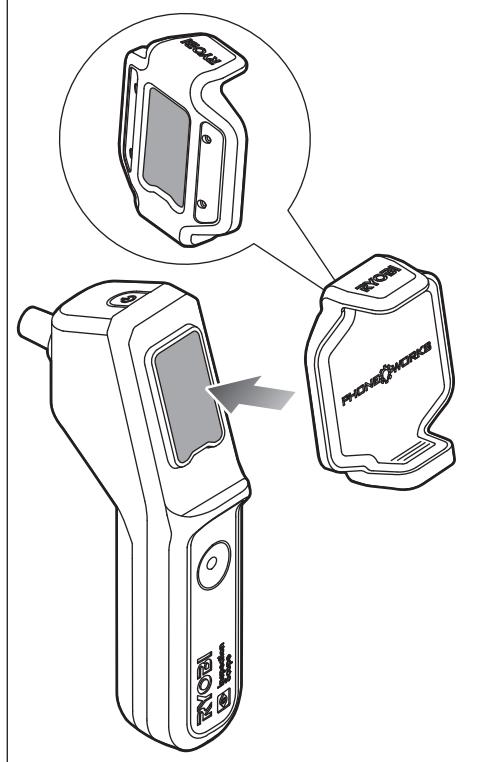
The clip expands to fit most smartphones. Always install the clip before attaching your smartphone.
